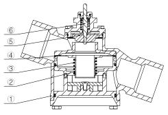
Materials: 1Valve Body: Ductile Iron
